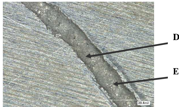
Photo 4. SEM wear groove view of a second Max5A tested sample.
