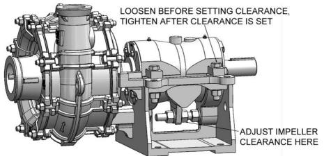
1. To set the impeller running clearance, first ensure the bearing cartridge clamp bolts are loose, then loosen the hex nuts (149B) on the bearing cartridge adjustment screw (149) located underneath the bearing cartridge (99) in the pedestal (53).
