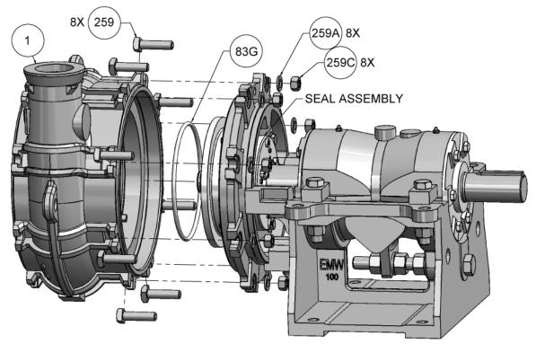
Case Assembly – Packing Seal
