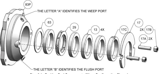
Step 6-1 - Packing Seal Components (Weep Configuration Shown)
