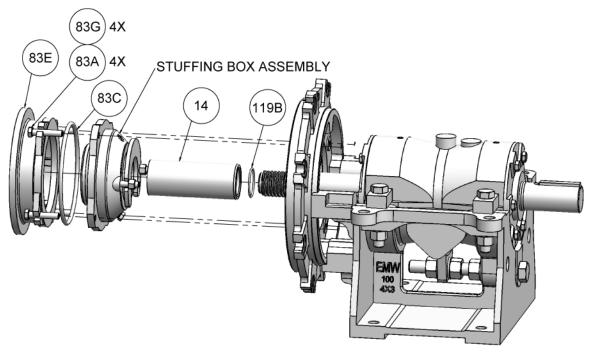
Packing Seal – Exploded View
