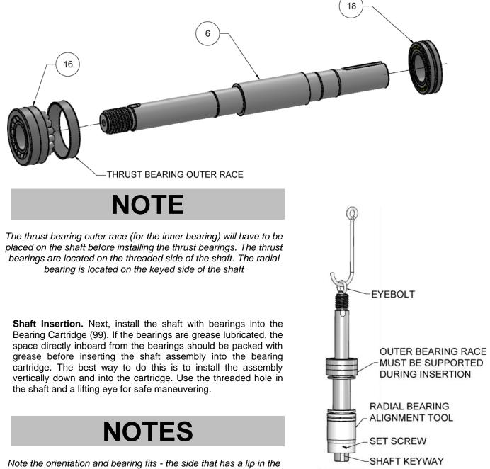
bore is the thrust bearing side (the side that the shaft is inserted into). Be careful when lowering the thrust bearing into the cartridge such that the outer races are inserted squarely.
