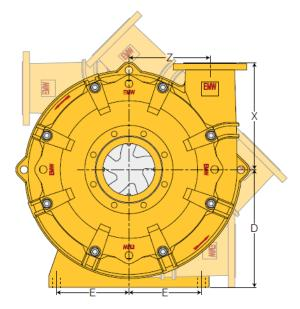
Pump with Direction of Rotation Arrow and optional case orientations
