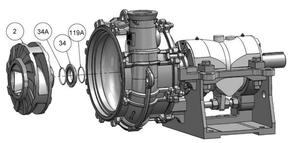
Impeller Installation – Packing Seal
