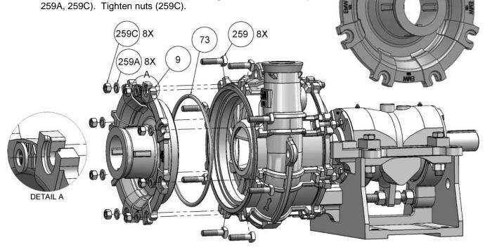
The arrow on the suction cover of the metal pump serves as position marker. Should an eccentric wear pattern develop, part life can be extended by clocking the suction cover to a new position. The arrow then provides a visual reference point identifying the clocking position. The arrow on the suction cover on factory supplied pumps will point upwards at the 12:00 position. When a new replacement is installed, the arrow should point upwards at the 12:00 position.
