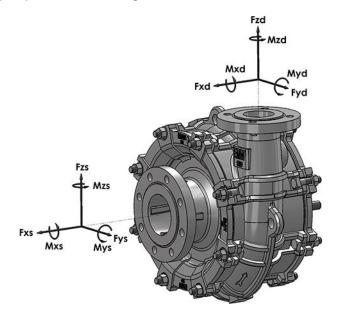
Note: Discharge nozzle coordinate system always moves with nozzle angle, Fz always moves in direction of flow.
