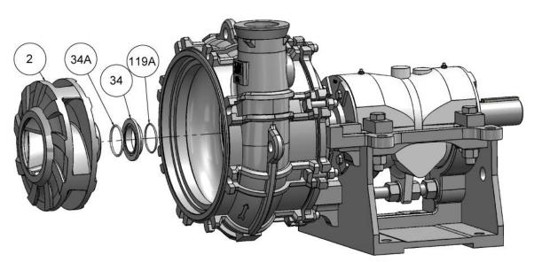
Impeller Assembly – Mechanical Seal
