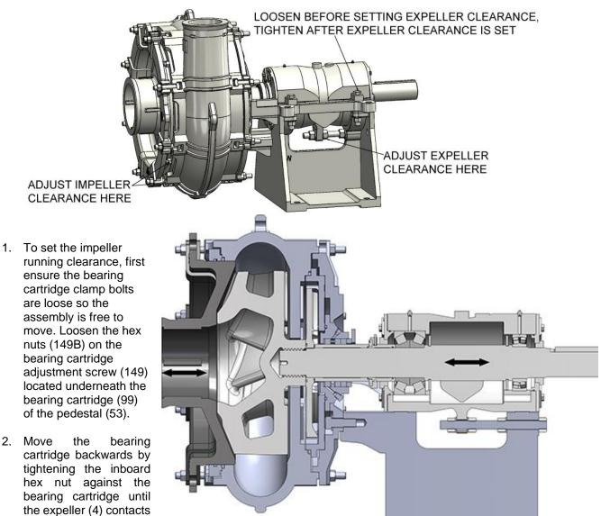
the expeller cover (71B). While making this adjustment, slowly rotate the shaft (6) to listen for rubbing. Then loosen the nut again to allow for frame travel.
