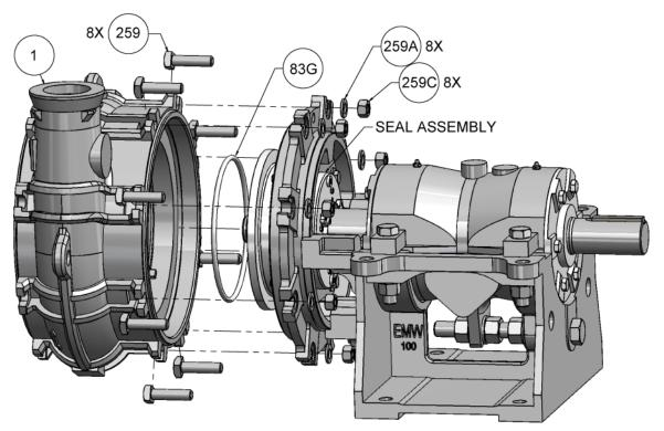
Case Assembly – Mechanical Seal
