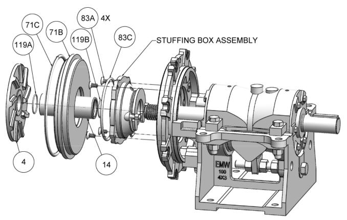
Expeller with Packing Seal – Exploded View
