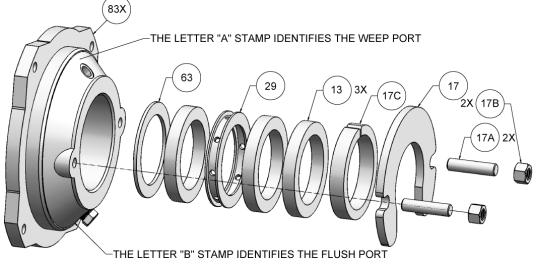
Expeller with Packing Seal Components (Weep Configuration Shown)
