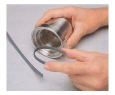
2. Insert the lip seal (25) into the rotary seal housing (24). Be sure the internal spring of the seal faces out. The seal (25) must seat completely in the groove of the rotary seal housing (24).
