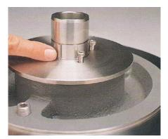
14. Place the ball housing assembly over the shaft sleeve (39) and secure with retaining ring (39A). Be sure the drive screws (24C) are seated in the holes of the ball housing (34). You may need to push down and compress the seal assembly to fit the retaining ring (39A) into its groove. A small block placed under the shaft sleeve (39) will help fully compress the assembly.
