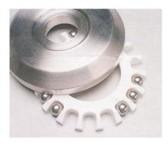
12. Attach the retaining ring (34A) to the hub of the ball housing (34).
