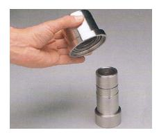
5. Carefully inspect the stationary seal ring (23) before installation. The inside surface of the seal ring (23) is the stationary seal face and must be free of scratches or nicks. Install the stationary seal ring (23) onto the rotary seal housing (24). Be careful not to damage the lip of the seal. The seal lip must seat on the widest diameter at the end of the housing (24).
