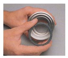
a. Check to make sure the seal groove in the rotary seal housing (24) is free of debris.
