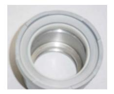
e. Make sure the excluder shaft seal (25) is centered in the rotary seal housing (24). The shaft sleeve (39) can be used to fully seat the seal.
