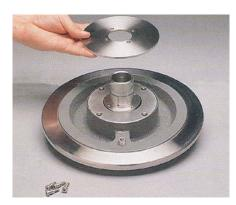
Place the balls (40A) into the slots of the ball retainer (40). For smooth operation, the balls (40A) must be symmetrically placed. Please note the small hole on the face of the ball retainer. This hole will fit over the spring pin (34B) in the ball housing (34).
