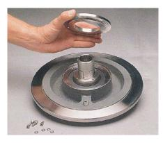
Attach the actuator (43) to the top of the rotary seal housing (24). Be sure the drive screws (24C) and drive nuts (24D) are securely tightened, and use Loc-Tite<sup>®</sup> 261 or its equivalent on the threads.
