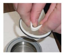
c. Position the large radius of the excluder shaft seal (25) in the rotary seal housing (24). Please note: the excluder shaft seal is not symmetrical. Make sure the step of the seal (25) is orientated so it is located over the short leg of the seal groove in the rotary seal housing (24).
