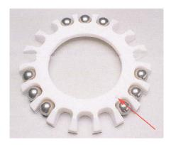
Set the ball housing (34) on top of the ball retainer (40). Be sure the spring pin (34B) is installed and fits into the hole of the ball retainer (40). Turn the assembly over.
