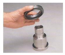
6. Place the backup seal (28) (which ever type that was supplied) onto the top of the stationary seal ring (23). (Note: if using a lube seal, pack with grease before installing on the stationary seal ring.)
