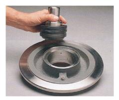
Attach the seal retainer (26) to the seal housing (30). Lock washers (26A) must be used with cap screws (26B). Be sure the cap screws (26B) are securely tightened.
