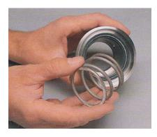
4. Slide the rotary seal housing (24) over the shaft sleeve (39). Carefully push the sleeve (39) past the slide rings and the lip seal. The rotary seal housing (24) must fit completely over the shaft sleeve (39). Install the shaft o-ring (20) into the groove in the shaft sleeve (39).
