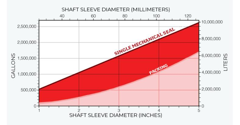
Charts are based on a pump running for 24 hours a day, 365 days a year. Solution contains 10-20% fine solids by weight. Data is based on best case scenario.
