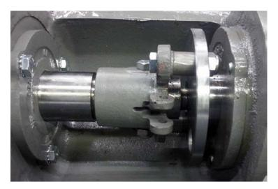
4. Remove the rotary seal (9) and gasket (10A) from the impeller (8).
