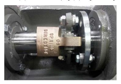
3. Lock the shaft using bushings (98M) and bolts (98L).
