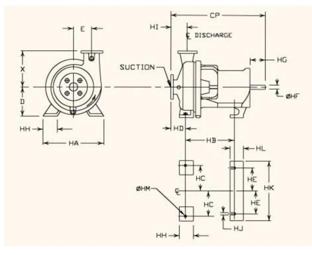
Dimensions shown are not for construction unless certified. Dimensions are shown in inches. Field shimming by customer may be required to meet dimensions. Baseplate dimensions are for fabricated steel.
