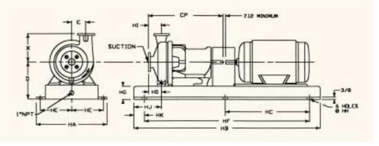
Dimensions shown are not for construction unless certified. Dimensions are shown in inches. Field shimming by customer may be required to meet dimensions. Baseplate dimensions are for fabricated steel.
