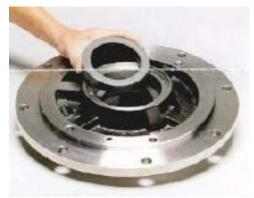
6. Place the backup seal (28) (which ever type that was supplied) onto the top of the stationary seal ring. (Note: if using a lube seal, pack with grease before installing on the stationary seal ring.)
