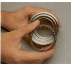
2. Insert the lip seal (25) into the rotary seal housing. Be sure the internal spring of the seal faces out. The seal must seat completely in the groove of the rotary seal housing.
