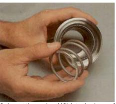
3. Insert the spring (42) into the bore of the rotary seal housing. Be careful not to damage the lip seal.
