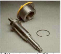
3. Slide the bearing carrier (72) onto outboard bearing and secure with retaining ring. Extreme duty bearings have a bearing plate that bolts to the bearing retainer instead of a retaining ring.
