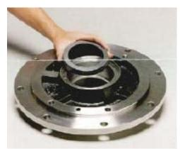
5. Carefully inspect the stationary seal ring (23) before installation. The inside surface of the seal ring is the stationary seal face and must be free of scratches or nicks. Lightly lubricate all seal orings to prevent damage. Install the stationary seal ring into the seal housing (30). Be careful not to damage the lip of the seal.
