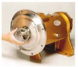
9. Install the barrier ring (35) to the hub of the rotary seal housing. The exposed metal insert faces away from the frame.
