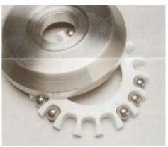
11. Set the ball housing on top of the ball retainer. Be sure the spring pin is installed and fits into the hole of the ball retainer. Turn the assembly over.
