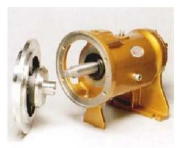
8. Install the seal assembly to the frame. Be careful not to damage the shaft o-ring during assembly. The top of the seal housing has two bosses and the bottom has only one.
