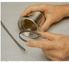
1. Place the slide rings (24A & 24B) into the bore of the rotary seal housing (24). The shortest slide ring goes into the rear of the housing.
