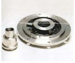
8. Slide the seal housing assembly over the shaft sleeve assembly, be careful not to damage the lips of the stationary seal.
