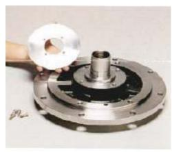
9. Attach the actuator (43) to the top of the rotary seal housing. The notch on the I.D. faces down. Be sure the drive screws (24C) and drive nuts (24D) are securely tightened, and use Loc-Tite® 261 or its equivalent on the threads.
