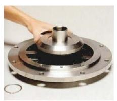
14. Place the ball housing over the shaft sleeve and secure with c-clip retaining ring (39A). Be sure the drive screws are seated in the holes of the ball housing. You may need to push down and compress the seal assembly to fit the retaining ring into its groove. A small block placed under the shaft sleeve will help fully compress the assembly.
