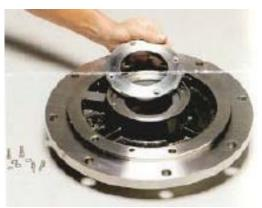
7. Attach the seal retainer (26) to the seal housing. Lock washers (26A) must be used with cap screws (26B). Be sure the cap screws are securely tightened.
