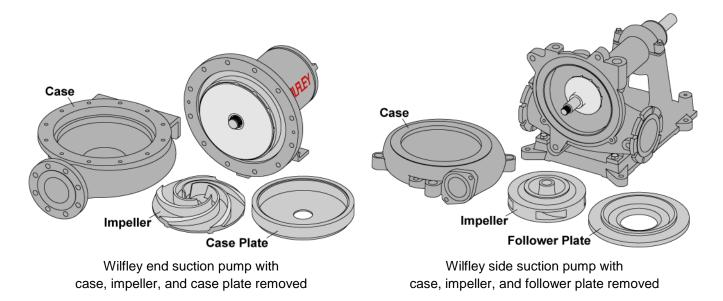
Returned pumps will be fully inspected by Wilfley and you will receive a proposal outlining the parts that need replacing and a schedule for completion. Once you agree to the proposal, the pump will be reassembled with new OEM parts and painted. A full range of optional performance tests are also available to meet your needs. All of the new OEM parts are furnished to you with a new pump warranty.
