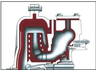
The draw bolt is provided to adjust for wear to maintain peak pump performance.
