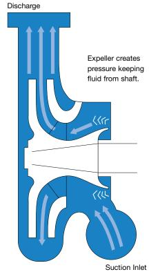
Impeller pumps fluid from intake to discharge
