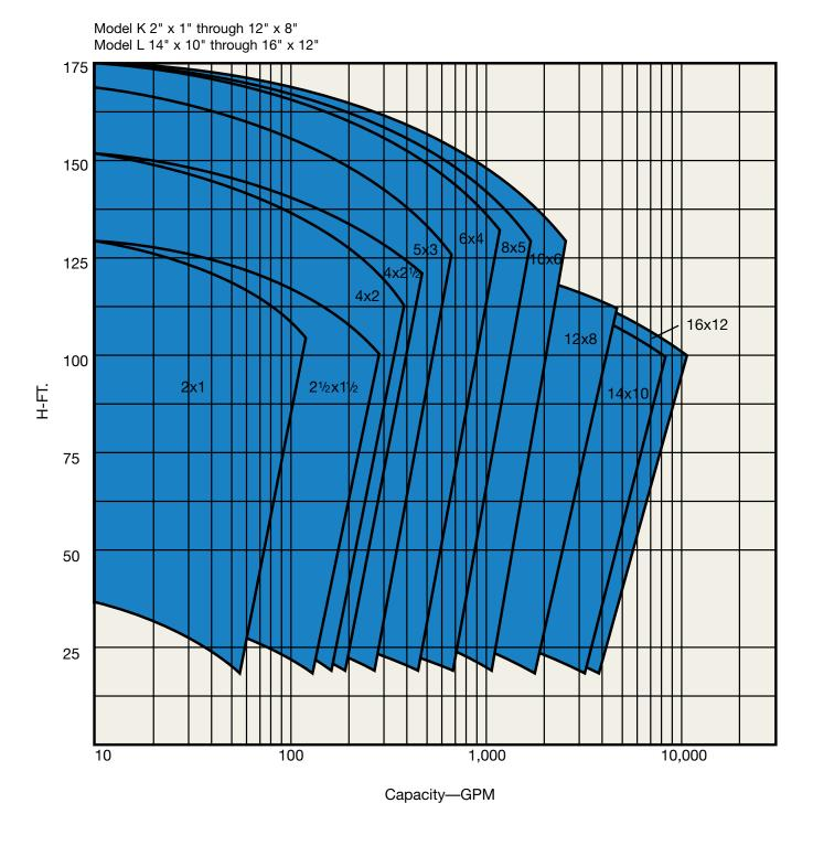
Model K pumps are available in discharge sizes ranging from 1" to 12". Cram arm assemblies that support the case during maintenance are available in discharge sizes 3" to 8". Larger pumps, designate model L use support base to slide the case away from the pump. Special pump configurations are available for high suction head and extreme horsepower services. Each pump is engineered to match service and system requirements.
