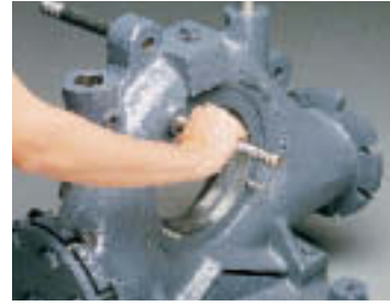
4. Install Gland Stud Bolts and the Draw Bolt on the back of the Intake Chamber.
