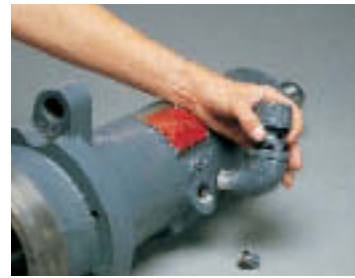
9. Install the Oil Filler Elbow assembly and the Oil Drain Plug on the Long Cylinder.
