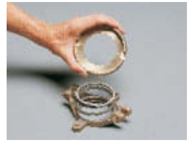
10. Place the Check Valve Spring into the Check Valve Spider and cover it with the Check Valve Packing Diaphragm Plate.
