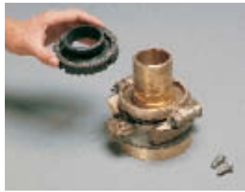
13. Slide the Check Valve Spider Assembly onto the Check Valve Sleeve, secure with screws. Position the Check Valve Packing Diaphragm on the Check Valve Packing Diaphragm Plate.
