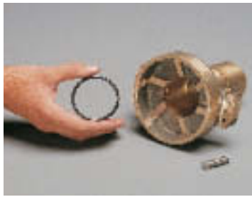
12. Install the Check Valve Setscrews and the Check Valve Sleeve O-Ring on the Check Valve Sleeve.
