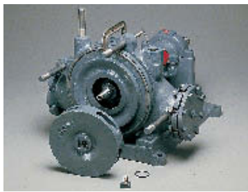
21. Slide Expeller O-Ring Runner onto the Shaft and secure with Runner Bolt. (Expeller O-Ring for two-piece Runner only). Note: C-Clamp may be useful in holding the Follower Plate in position.
