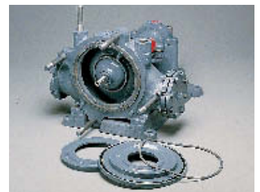
20. Install Frame Protecting Ring, Follower Plate and follower Plate Gasket into Front Bore of Intake Chamber.
