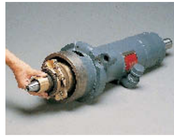
14. Slide the Check Valve Assembly onto the Shaft and tighten the Setscrew in the notch on the Shaft.
