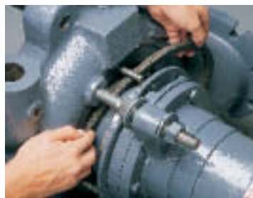
18. Install two layers of Gland Packing Ring into rear bore of the Intake Chamber and bolt the Gland Ring to the Intake Chamber. Attach Short Cylinder Cover. Do not tighten at this time.
