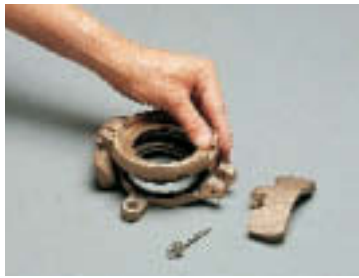
11. Compress the Check Valve Packing Diaphragm Plate and attach the Check Valve Weights with the cotter pins and washers.
