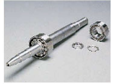
5. Heat Bearings and slide them onto the Bearing Shoulders on the Shaft. Lock into place with Lock Nuts and Lock Washers.
