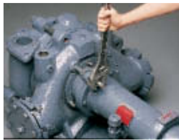
23. Set Runner Clearance. For specific instructions refer to page 5 of the Model K Operating Handbook. Tighten Pedestal Cap and Gland Stud Nuts.
