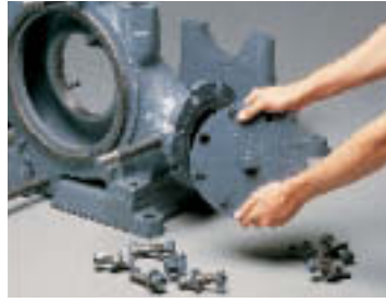
3. Bolt the Blind Intake Flange onto the Intake Chamber. Note: Wilfley Model K pumps will accept intake from either, or both sides of the pump.
