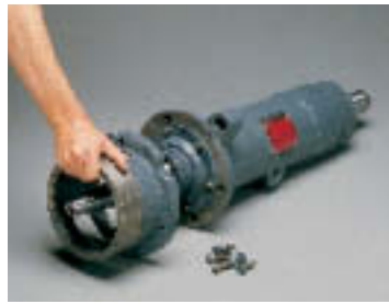
8. Attach short cylinder to the Long Cylinder. Note: dished edge of the Short Cylinder must line up with the Draw Bolt Fitting on the Long Cylinder.
