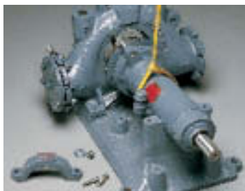
17. Install Bearing Unit in rear bore of Intake Chamber. Attach Pedestal Cap and Draw Bolt Nut and Washer. Do not tighten at this time.
