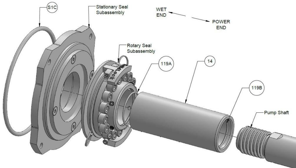
3. Install stationary seal o-ring (S1C) on to the wet end of the stationary seal. Apply lubrication to the o-ring as specified in the Solidlock® instruction manual **IM-SL**.
