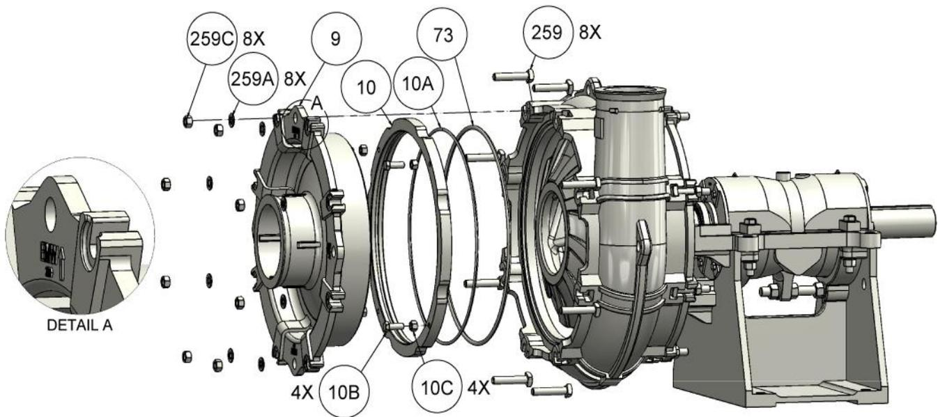
The arrow on the suction cover of the metal pump serves as position marker. Should an eccentric wear pattern develop, part life can be extended by clocking the suction cover to a new position. The arrow then provides a visual reference point identifying the clocking position. The arrow on the suction cover on factory supplied pumps will point upwards at the 12:00 position. When a new replacement is installed, the arrow should point upwards at the 12:00 position.
