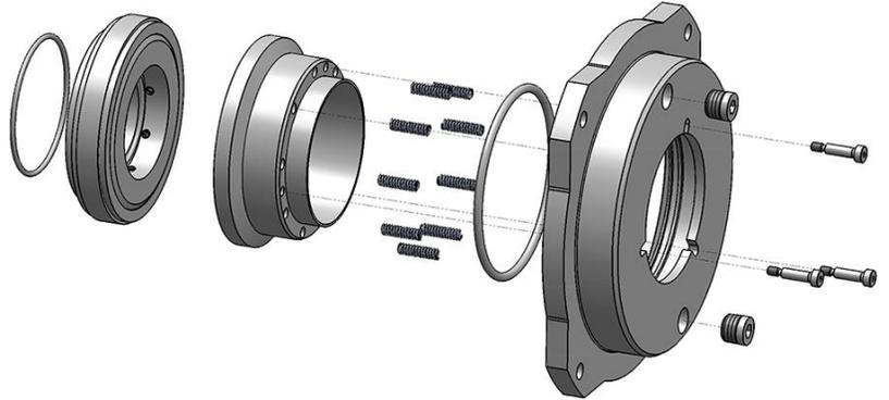
**Semi-Cartridge Style Mechanical Seal**
