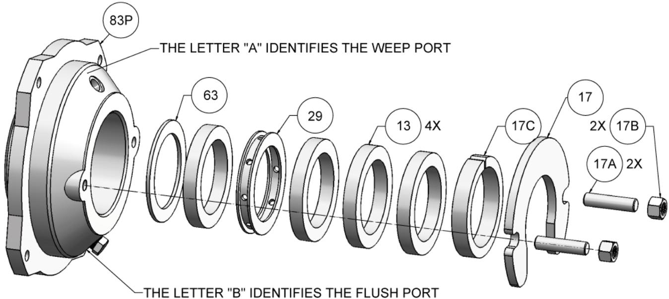
**Step 6-1 - Packing Seal Components (Weep Configuration Shown)**
