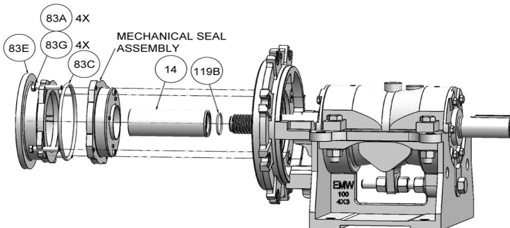
**Mechanical Seal Installation**
