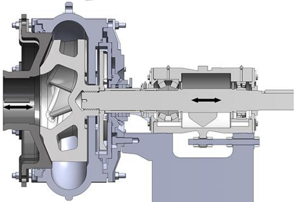
2. Move the bearing cartridge backwards by tightening the inboard hex nut against the bearing cartridge until the expeller (4) contacts the expeller cover (71B). While making this adjustment, slowly rotate the shaft (6) to listen for rubbing. Then loosen the nut again to allow for frame travel.
