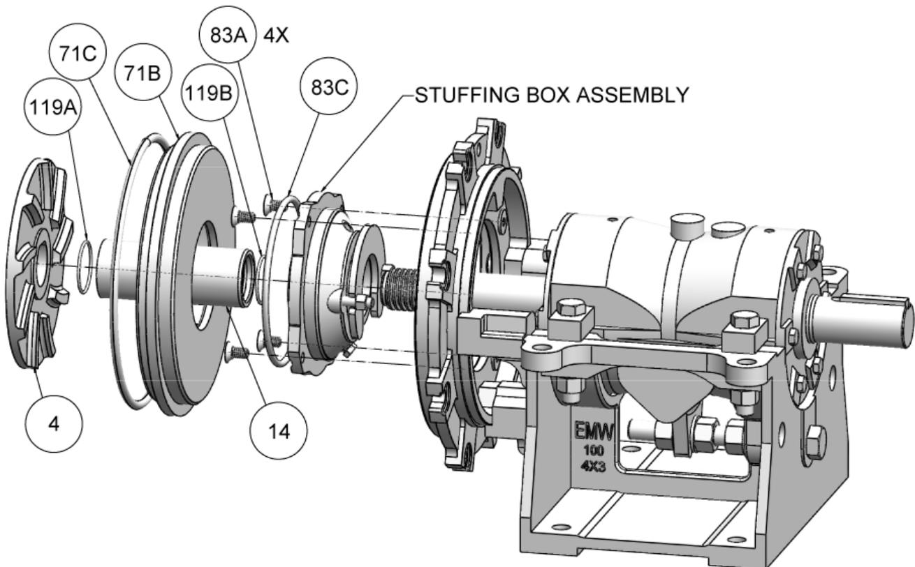
Expeller with Packing Seal – Exploded View
