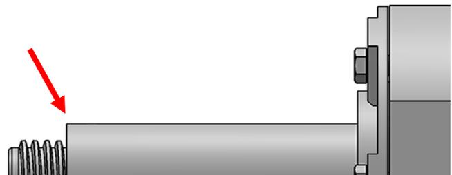
**Incorrectly installed shaft sleeve
