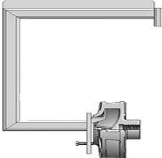
or from a bearing cartridge is required. A tool that shoulders against the radial bearing outer race, slip fits over the drive end of the shaft and is secured in the keyway by a set screw is recommended. To avoid damaging the shaft, the set screw should only be tightened against the shaft keyway flat.
