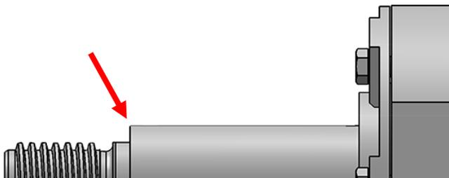
**Correctly installed shaft sleeve
