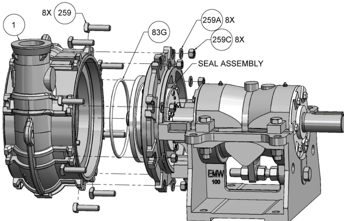
Case Assembly – Packing Seal
