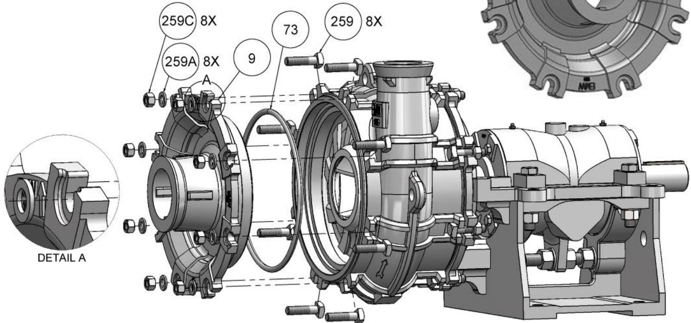
The arrow on the suction cover of the metal pump serves as position marker. Should an eccentric wear pattern develop, part life can be extended by clocking the suction cover to a new position. The arrow then provides a visual reference point identifying the clocking position. The arrow on the suction cover on factory supplied pumps will point upwards at the 12:00 position. When a new replacement is installed, the arrow should point upwards at the 12:00 position.
