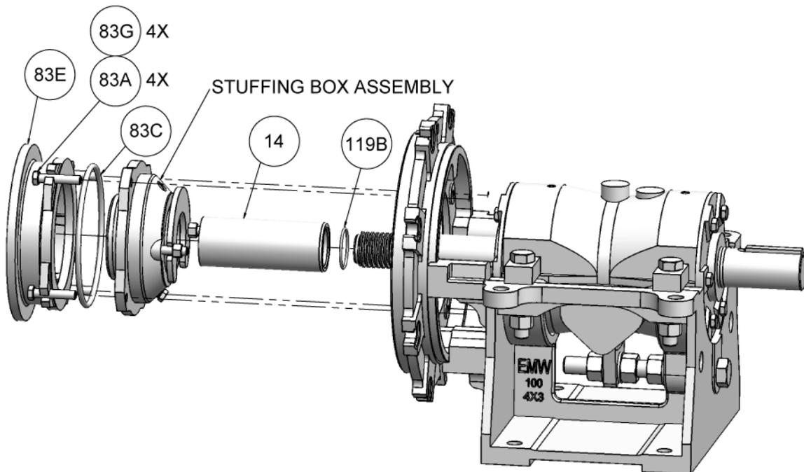
**Packing Seal – Exploded View**
