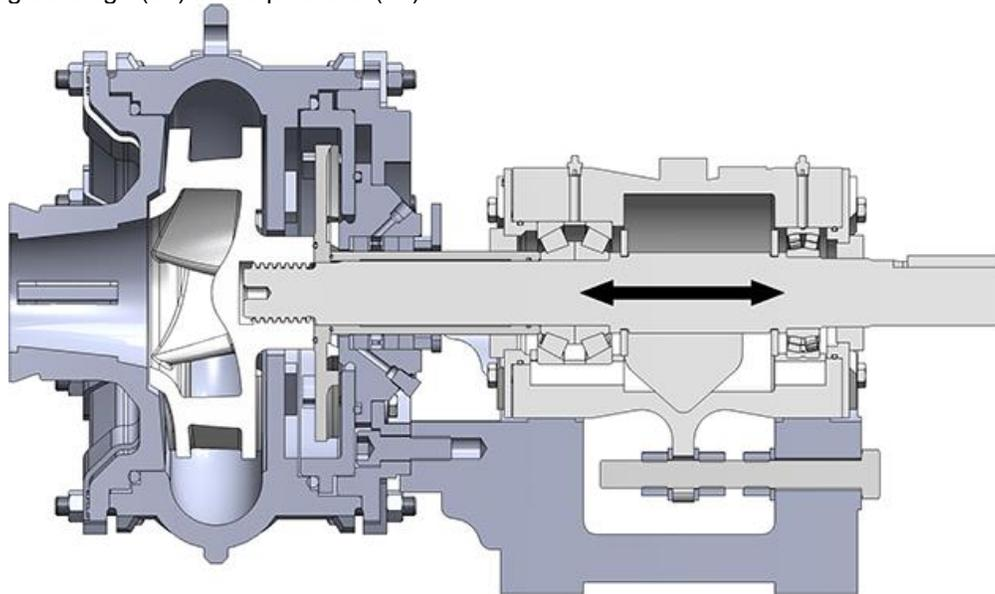
2. Move the bearing cartridge forward (left) using the outboard hex nut against the bearing cartridge adjustment screw until the impeller (2) contacts the suction cover (9).
