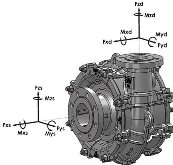
Note: Discharge nozzle coordinate system always moves with nozzle angle, Fz always moves in direction of flow.
