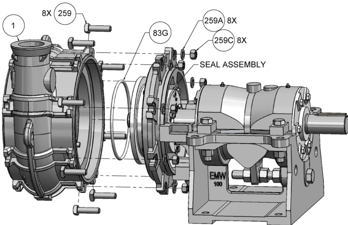
**Case Assembly – Mechanical Seal**
