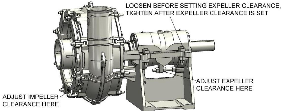
1. To set the impeller running clearance, first ensure the bearing cartridge clamp bolts are loose so the assembly is free to move. Loosen the hex nuts (149B) on the bearing cartridge adjustment screw (149) located underneath the bearing cartridge (99) of the pedestal (53).
