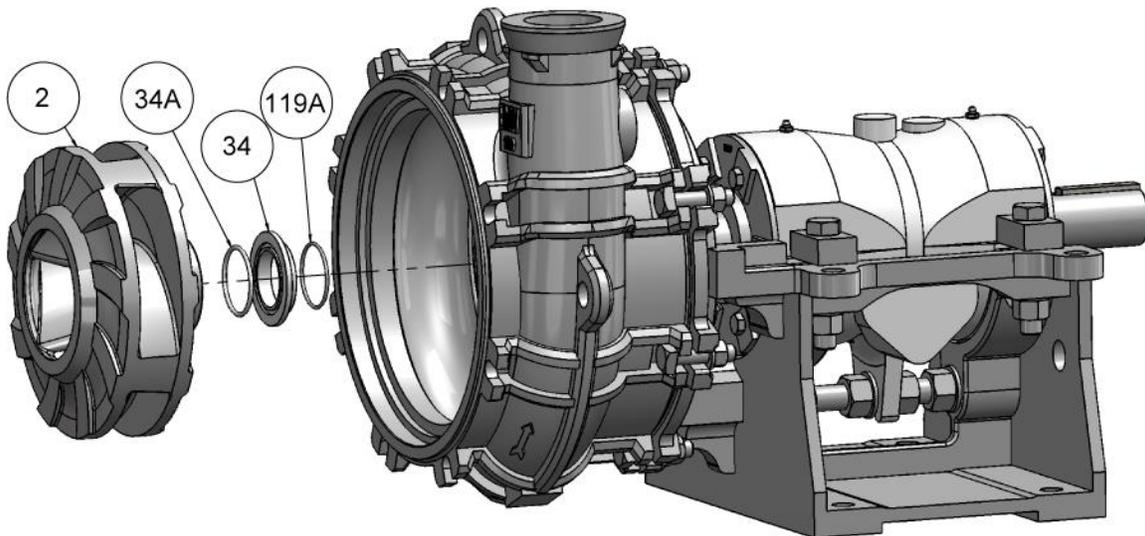
**Impeller Installation – Packing Seal**
