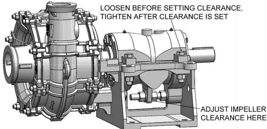
1. To set the impeller running clearance, first ensure the bearing cartridge clamp bolts are loose, then loosen the hex nuts (149B) on the bearing cartridge adjustment screw (149) located underneath the bearing cartridge (99) in the pedestal (53).
