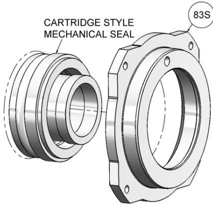
**Cartridge Style Mechanical Seal**
