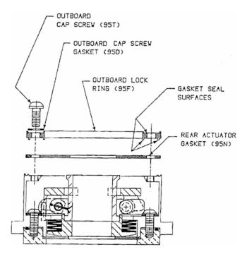
THE HYDROVOIR IS NOW READY TO BE ASSEMBLED INTO A WILFLEY MODEL AF PUMP. PLEASE REFER TO HYDROVOIR INSTALLATION INSTRUCTIONS, PAGE 15, TO COMPLETE PUMP ASSEMBLY.
