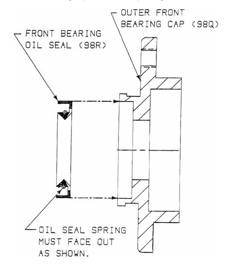
11. Grease the oil seal lip, carefully slide the outer front bearing cap (98Q) onto the shaft and secure to the frame (19) using the bearing cap screws and lockwashers (18B,C). Be very careful not to damage the lip of the seal during assembly.
