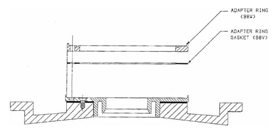
4. Place the reservoir expeller (96F) into the cavity of the hydrovoir labyrinth ring (98G) with the vanes facing up. Insert the reservoir o-ring (96E) into its groove in the adapter ring (Frames 1 and 2) or the hydrovoir labyrinth ring. Lubricate the o-ring with grease to hold it in place during assembly.
