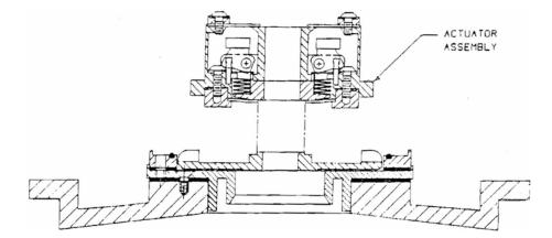
6. Place the reservoir (96B) over the actuator assembly and bolt to the hydrovoir labyrinth ring (98G). Frame 3 and 4 have an uneven bolt pattern on the reservoir with three holes around the upper half and four in the lower or flat side of the reservoir. Frame 1 and 2 require adapter ring flat washers (98T) underneath the labyrinth lockwashers (96Q).
