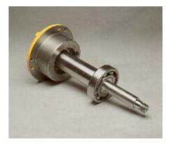
4. Install the inboard bearing (62A) onto the shaft.
