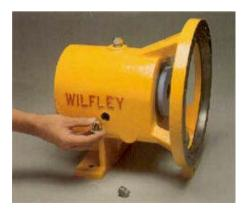
6. Install the breather (61A), sight glass (79), and drain plug (61B) into the frame.
