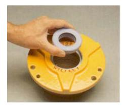
2. Install the outboard oil seal (76) into the bearing carrier (72). Please be sure that the notch in the seal faces down for drainage.
