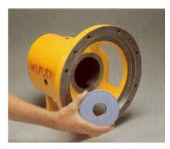
5. Install the inboard oil seal (67) into the frame.
