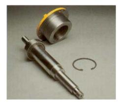
3. Slide the bearing carrier over the shaft and outboard bearing, and install the retaining ring (73) into the groove of the bearing carrier. Be sure the retaining ring is fully seated in the groove.
