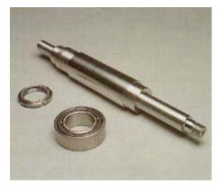
Install the outboard bearing (62B) and locknut (62C) onto the shaft (62). We recommend that a bearing heater be used when installing bearings to avoid damage to the races. Be sure the bearing seats against the shoulder of the shaft. If the pump is grease lubricated, hand pack the bearings with the appropriate grease after the bearings are seated on the shaft.
