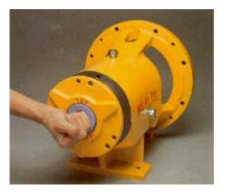
7. Install the bearing carrier o-ring (72A) into the groove of the bearing carrier. To avoid damage, lubricate the o-ring with light oil and slide the assembly into the frame. The word "top" on the carrier must face up. Attach the bearing carrier with three retaining bolts (75), jacking bolts (75), and jam nuts (72B).
