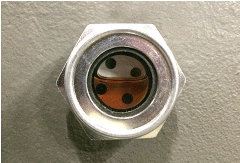
Oil site glass showing the appropriate amount of oil.
