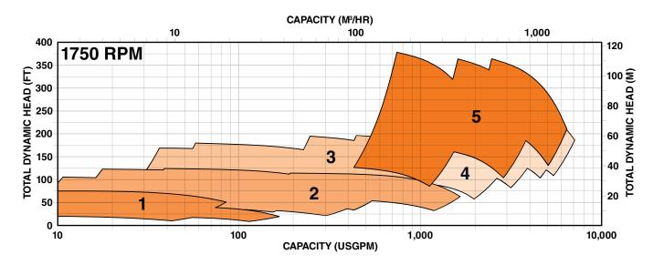
The Frame 5 A9 can deliver up to an impressive 6,000 USgpm (1,350 m<sup>3</sup>/hr) and 400 feet (120m).
