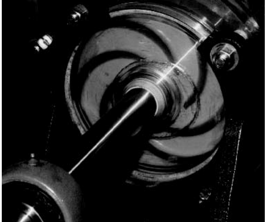
Wilfley hydraulic seal in actual operation.
